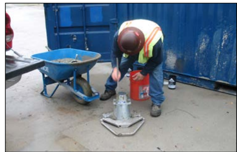
performing concrete slump test
