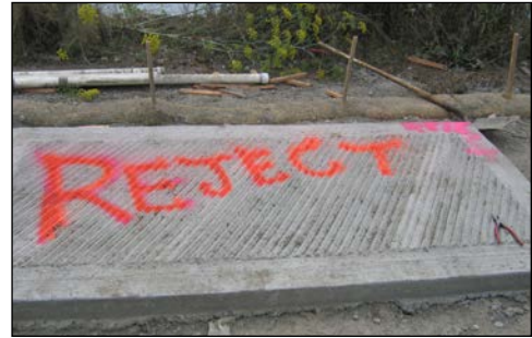
rejected V-groove test panel
