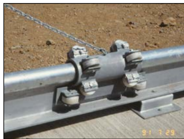
trolley is made of a slotted steel pipe with multiple types of wheels attached to pipe-rail and trolley
