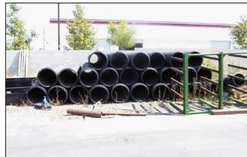
circular pontoons to be foam filled
