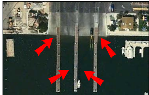
8 lane launching ramp with 2 pairs of three adjacent boat launching lanes bordered by 2 single lanes
